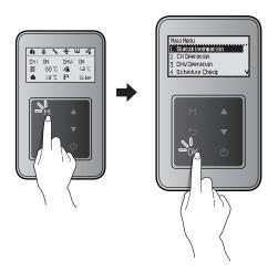
Press the Up button ( $\blacktriangle$ ) or the Down button ( $\blacktriangledown$ ) to switch between the information items. Press the OK button ( $\bigcirc$ K) to select an item and view the information.
