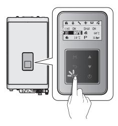
3. Press the Up button (▲) or the Down button (▼) until the desired temperature appears on the display. You can adjust the temperature while the display is flashing. Once the display stops flashing, the temperature setting is stored.
