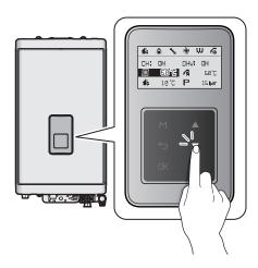
2. Press the OK button (○K) to select the central heating temperature (Ⅲ). The highlighted section will flash.
