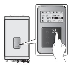
3. Press the OK button (○K) to select the DHW temperature (♠). The highlighted section will flash.
