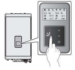
If resetting the boiler and attempting the remedies suggested below do not resolve the problem, contact the Technical Helpdesk or a Gas Safe Registered Engineer.
