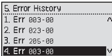
Press the Up button (▲) or the Down button (▼) to switch between the list of Errors. Press the OK button (OK) to select an error to view detailed information.
