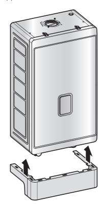
3. Remove the two screws at the bottom of the boiler.
