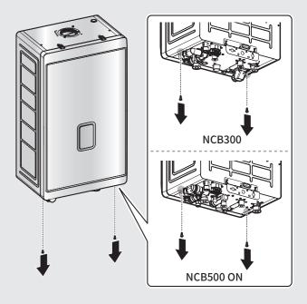
5. Properly align the pipe cover with the bottom of the boiler, and then fasten the two screws (previously removed from the boiler) or use spare screws to secure the pipe cover to the boiler.
