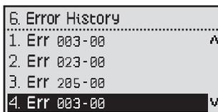
Rotate the Command dial (⊙) to switch between the list of errors. Press the Command dial (⊙) to select an error to view detailed information.
