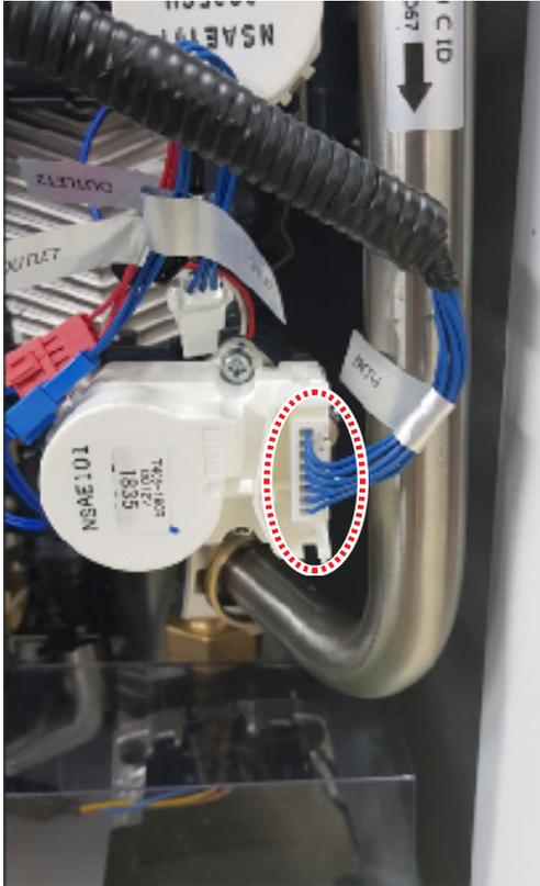
4. Remove the 2 clips fixing the flow control valve.
