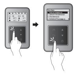
Press the Up button ( $\blacktriangle$ ) or the Down button ( $\bigtriangledown$ ) to switch between the information items. Press the OK button ( $\bigcirc$ K) to select an item and view the information.
