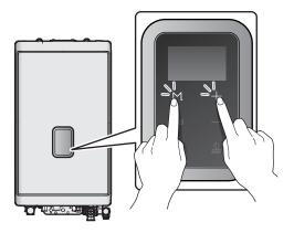
Press the ECO button (<c $\varnothing$ ). The CH Heat Demand blinks on the screen. Then, press the Plus button (+) or the Minus button (-) to set the CH Heat Demand. Press the ECO button (<c $\varnothing$ ) to save the value.
