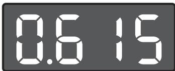
Press the Plus button (+) or the Minus button (-) to switch between the list of Errors. Press the ECO button (εε∅) to select an error to view the elapsed time since the last error occurred.
