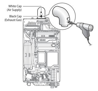
Figure 7. Insert the Analyser
