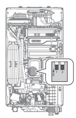
Figure 6. Set the DIP switches
