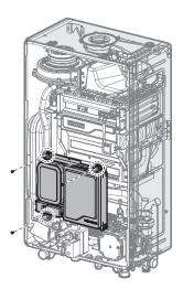
7. Remove the front panel assembly.
