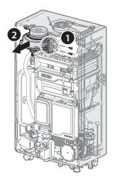
9. Remove the four bolts securing the chamber brackets.
