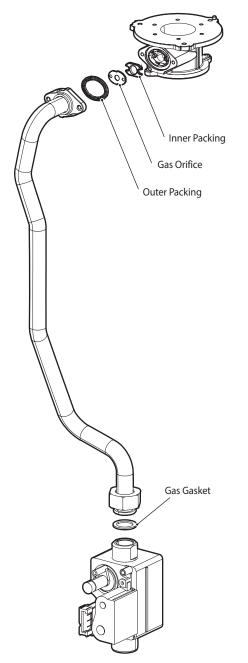
Figure 5.2. Exploded View of Gas Pipe Assembly (NCB300-37K, NCB300-41K)
