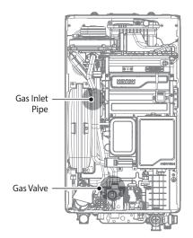
Figure 2. NCB300 Internal Components
