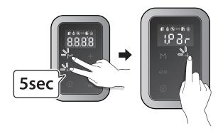
In the password screen, press the Plus button (+) or the Minus button (-) to change numbers and places, and press the ECO button ( $\leq c \sigma$ ) to enter the password.
