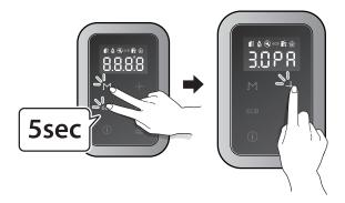
Press the Plus button (+) or the Minus button (-) to switch between the operation modes. Press the ECO button ( $\in CO$ ) to select an operation mode.
