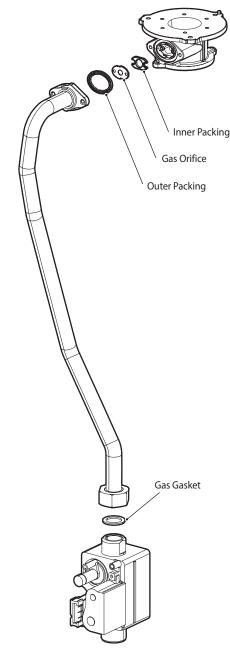
Figure 5.1. Exploded View of Gas Pipe Assembly (NCB300-28K)
