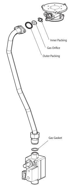
Figure 5. Exploded View of Gas Pipe Assembly (NCB500)
