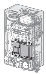
7. Remove the front panel assembly.
