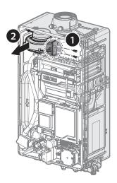
9. Remove the four bolts securing the chamber brackets.
