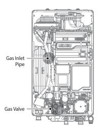
Figure 2. NCB500 Internal Components
