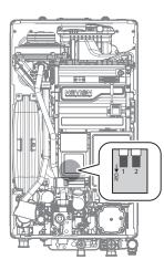
Figure 6. Set the DIP switches
