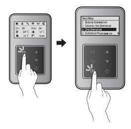
Press the Up button (  $\blacktriangle$  ) or the Down button (  $\blacktriangledown$  ) to switch between the list items or to increase/decrease setting values. Press the OK button (OK) to select an item or to confirm after making changes.
