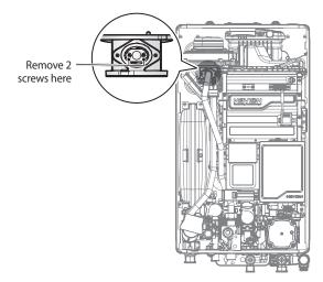
Figure 4. Access to Gas Orifice in Fan Assembly
