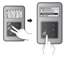
On the password screen, press the Up button ( $\blacktriangle$ ) and the Down button ( $\blacktriangledown$ ) to change numbers and places, and press the OK button (OK) to enter the password. The factory default password is "1234".
