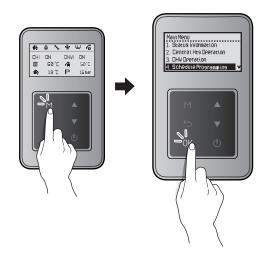
Press the Up button (  $\blacktriangle$  ) or the Down button (  $\triangledown$  ) to switch between the list items or to increase/decrease setting values. Press the OK button (OK) to select an item or to confirm after making changes.
