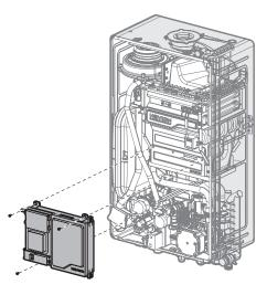
8. With the internal components exposed, locate the gas inlet pipe and the gas valve in the middle of the unit, as shown in Figure 2.
