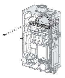
10. Remove the rubber packing at the top of the cover and put a Phillips screwdriver into the hole, and then loosen the middle bolt located at the back of the burner.
