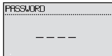
After entering the parameter setting screen, press the Up button (▲) or the Down button (▼) to switch between the parameters or to increase/decrease setting values. Press the OK button (OK) to select a parameter or to confirm after making changes.
