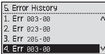
Press the Up button (▲) or the Down button (▼) to switch between the list of Errors. Press the OK button (OK) to select an error to view detailed information.
