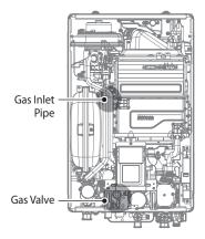
Figure 2-1. NCB700-2S+/42K Internal Components
