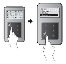
Press the Up button ( $\blacktriangle$ ) or the Down button ( $\blacktriangledown$ ) to switch between the list items or to increase/decrease setting values. Press the OK button (0K) to select an item or to confirm after making changes.
