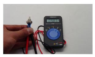
Check if the hot water temperature sensor is open (Error type:  $\mbox{M}\Omega$  Open)
