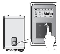
Press the OK button (○K) to select the DHW temperature (★). The highlighted section will flash.
