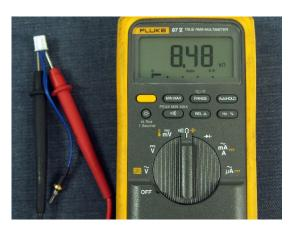
Test to confirm if the hot water temperature sensor is open. Error:  $\mbox{M}\Omega$  open circuit.
