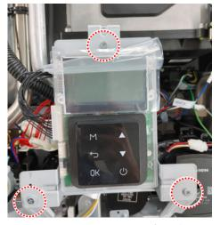
Figure 13 Disconnect wiring connector from the main PCB.
