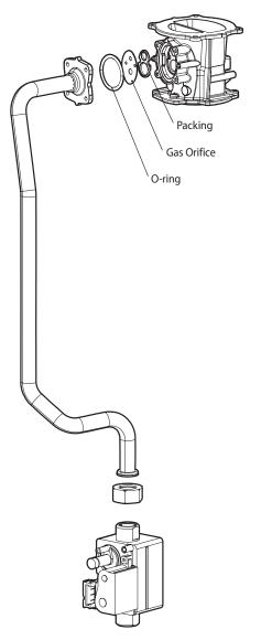
Figure 5-2. Exploded View of Gas Pipe Assembly (NCB700-3S/54K)
