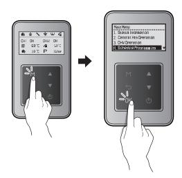
Press the Up button ( $\triangle$ ) or the Down button ( $\nabla$ ) to switch between the list items or to increase/decrease setting values. Press the OK button (OK) to select an item or to confirm after making changes.
