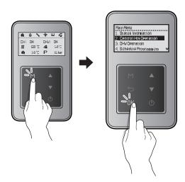
Press the Up button ( $\triangle$ ) or the Down button ( $\nabla$ ) to switch between the list items or to increase/decrease setting values. Press the OK button (0K) to select an item or to confirm after making changes.
