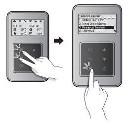
In the password screen, press the Up button ( $\triangle$ ) or the Down button ( $\nabla$ ) to change numbers and places, and press the OK button ( $\bigcirc$ K) to enter the password.
