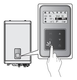
4. Press the Up button (▲) or the Down button (▼) until the desired temperature appears on the display. You can adjust the temperature while the display is flashing. Once the display stops flashing, the temperature setting is stored.
