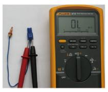
Test to confirm if the secondary water temperature sensor is open. Error:  $M\Omega$  open circuit.
