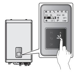
2. Press the OK button (○K) to select the central heating temperature (Ⅲ). The highlighted section will flash.
