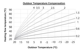
If there is an input from the outdoor temperature sensor, OTC (Outdoor Temperature Compensation) control will be enabled automatically. Also, if there is no input from the outdoor temperature sensor, OTC control will be disabled automatically.
