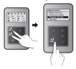
On the password screen, press the Up button ( $\triangle$ ) and the Down button ( $\nabla$ ) to change numbers and places, and press the OK button (0K) to enter the password.
