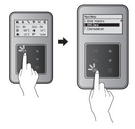
Press the Up button ( $\blacktriangle$ ) or the Down button ( $\blacktriangledown$ ) to switch between the information items. Press the OK button (0K) to select an item and view the information.
