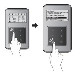
Press the Up button ( $\blacktriangle$ ) or the Down button ( $\blacktriangledown$ ) to switch between the list items or to increase/decrease setting values. Press the OK button (0K) to select an item or to confirm after making changes.
