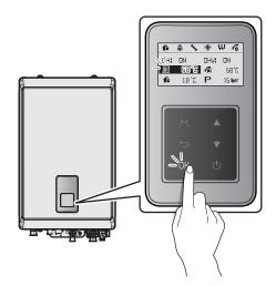
Press the Up button (▲) or the Down button (▼) until the desired temperature appears on the display. You can adjust the temperature while the display is flashing. Once the display stops flashing, the temperature setting is stored.
