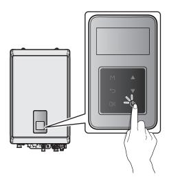
When the power is turned on for the first time, you must complete the set-up wizard. The temperature will appear on the front panel display after the power is turned on.
