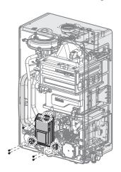
7. Remove the front panel assembly.
