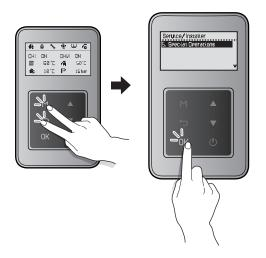
Press the Up button ( $\blacktriangle$ ) or the Down button ( $\blacktriangledown$ ) to switch between the operation modes. Press the OK button (ОK) to select an operation mode.
