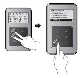
Press the Up button ( $\triangle$ ) or the Down button ( $\nabla$ ) to switch between the test procedures. Press the OK button ( $\overline{OK}$ ) to run a test procedure.
