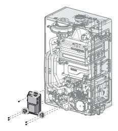
8. With the internal components exposed, locate the gas inlet pipe and the gas valve in the middle of the unit, as shown in Figure 2-1 and Figure 2-2.
