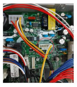
Check the voltage at the solenoid valve / Yellow - White
