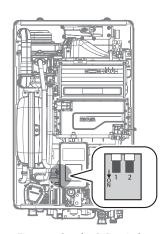
Figure 6. Set the DIP switches
