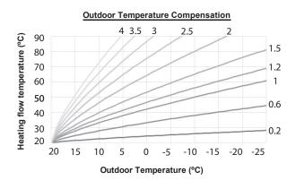
If there is an input from the outdoor temperature sensor, OTC (Outdoor Temperature Compensation) control will be enabled automatically. Also, if there is no input from the outdoor temperature sensor, OTC control will be disabled automatically.
