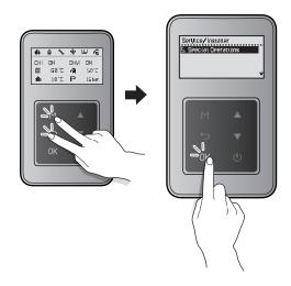
Press the Up button (  $\blacktriangle$  ) or the Down button (  $\blacktriangledown$  ) to switch between the operation modes. Press the OK button (OK) to select an operation mode.
