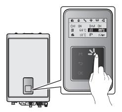
3. Press the OK button (OK) to select the DHW temperature (A). The highlighted section will flash.
