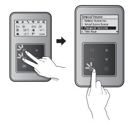
In the password screen, press the Up button (  $\blacktriangle$  ) or the Down button (  $\blacktriangledown$  ) to change numbers and places, and press the OK button (OK) to enter the password.
