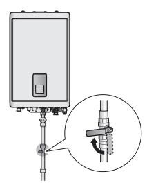
6. Close off any heating zones that do not require draining and open a purge valve to drain the central heating side. Open all domestic hot water taps completely to drain the water heating side. The water that remains in the plumbing lines will drain out.
