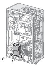
7. Remove the front panel assembly.
