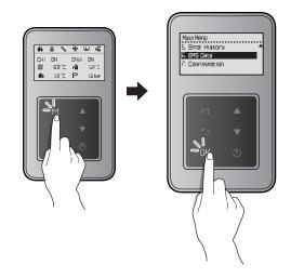
Press the Up button (  $\blacktriangle$  ) or the Down button (  $\triangledown$  ) to switch between the information items. Press the OK button ( $\bigcirc$ K) to select an item and view the information.
