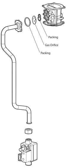
Packing Gas Orifice O-ring
