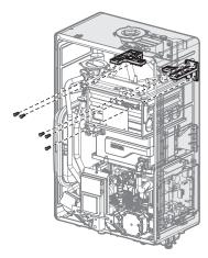
Remove the two screws connecting the ignition transformer to the heat exchanger and then remove the ignition transformer.
