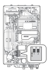
Figure 6. Set the DIP switches
