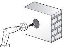
ø105 mm for terminal ø60/100 mm ø130 mm for terminal ø80/120 mm
