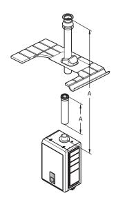
Ø60/100 => Max. length: A=21 m Ø80/125 => Max. length: A=70 m
