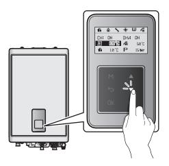
Press the OK button (○K) to select the central heating temperature (IIII). The highlighted section will flash.
