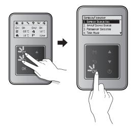
Press the Up button (  $\blacktriangle$  ) or the Down button (  $\triangledown$  ) to switch between the information items. Press the OK button (OK) to select an item and view the information.
