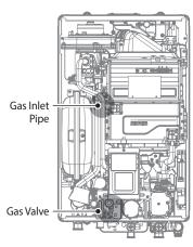
Figure 2-1. NCB700-2S+/42K Internal Components
