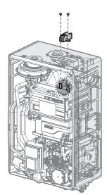
11. Remove the rubber packing at the top of the cover and put a Phillips screwdriver into the hole, and then loosen the middle bolt located at the back of the burner.
