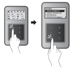
Press the Up button ( $\blacktriangle$ ) or the Down button ( $\bigtriangledown$ ) to switch between the information items. Press the OK button ( $\bigcirc$ K) to select an item and view the information.
