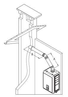
Ø60/100 => Max. length: A+B-(1 x 45°elbow) = 20-1.2=18.8 m Ø80/125 => Max. length: A+B-(1 x 45°elbow) = 68-1.2=66.8 m
