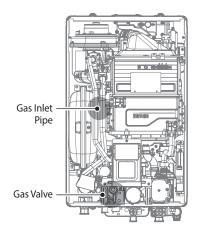
Figure 2-2. NCB700-3S/54K Internal Components
