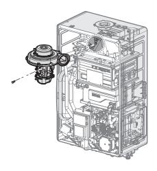
9. Remove the five bolts securing the chamber brackets.
