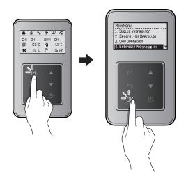
Press the Up button (  $\blacktriangle$  ) or the Down button (  $\blacktriangledown$  ) to switch between the list items or to increase/decrease setting values. Press the OK button (OK) to select an item or to confirm after making changes.
