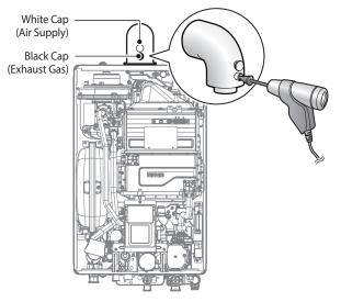
Figure 7. Insert the Analyser
