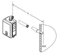
Ø60/100 => Max. length: A=20 m Ø80/125 => Max. length: A=68 m
