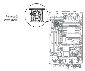
Figure 4. Access to Gas Orifice in Fan Assembly
