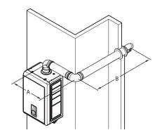
Ø60/100 => Max. length: A+B-(1 x 90°elbow) = 20-2.4=17.6 m Ø80/125 => Max. length: A+B-(1 x 90°elbow) = 68-2.4=65.6 m
