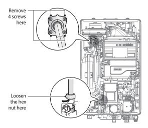
8. Remove the screw connecting the fan motor assembly and the mixing chamber, and then remove the fan motor assembly.
