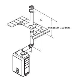
Ø60/100 => Max. length: A+B-(1 x 45°elbow) = 21-1.2=19.8 m Ø80/125 => Max. length: A+B-(1 x 45°elbow) = 70-1.2=68.8 m
