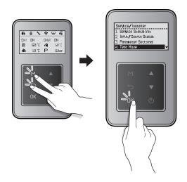
Press the Up button (  $\bigstar$  ) or the Down button (  $\blacktriangledown$  ) to switch between the test procedures. Press the OK button (OK) to run a test procedure.
