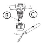
3. Insert cable "C" into the lid "A" together with the seal "B".
