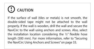
If the wall cannot be drilled, secure the NaviCirc to the wall using the bracket with a double-sided tape and primer.
