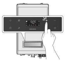
You can adjust the temperature while the display is flashing. If no buttons are pressed for 5 seconds or if the INFO button is pressed, the current temperature setting will be stored automatically.
