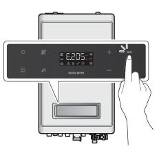
If resetting the boiler does not solve the problem, refer to the Troubleshooting section of this manual or contact a Technical Assistance Service.
