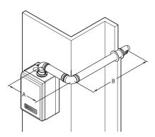
$\emptyset$ 60/100 => Max. length: A+B-(1 x 90°elbow) = 20-1.3 = 18.7 m  $\emptyset$ 80/125 => Max. length: A+B-(1 x 90°elbow) = 68-2.2 = 65.8 m
