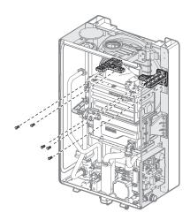
Remove the two screws connecting the ignition transformer to the heat exchanger and then remove the ignition transformer.
