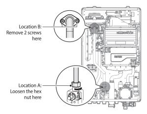
Figure 3-1. Detaching Gas Inlet Pipe from Gas Valve and Fan Motor Assembly (NCB-24/28/34LDWE)
