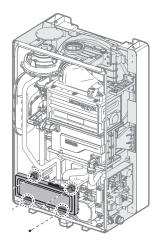
7. Remove the PCB assembly.
