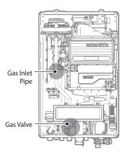
Figure 2-1. NCB-24/28/34LDWE Internal Components
