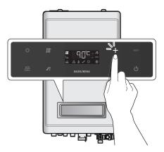
You can adjust the temperature while the display is flashing. If no buttons are pressed for 5 seconds or if the ECO button is pressed, the current temperature setting will be stored automatically.
