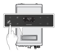
Press the + (Up) or - (Down) buttons to switch between the information types.
