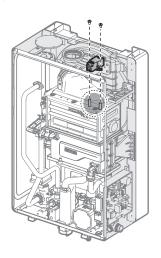
11. Remove the rubber packing at the top of the cover and put a Phillips screwdriver into the hole, and then loosen the middle bolt located at the back of the burner.
