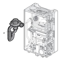
9. Remove the five bolts securing the chamber brackets.
