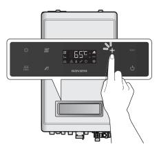
You can adjust the temperature while the display is flashing. If no buttons are pressed for 5 seconds or if the ECO button is pressed, the current temperature setting will be stored automatically.
