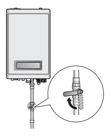
6. Close off any heating zones that do not require draining and open a purge valve to drain the space heating side. Open all domestic hot water taps completely to drain the water heating side. The water that remains in the plumbing lines will drain out.
