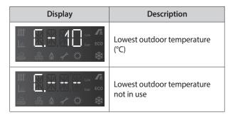
This mode is used to configure the lowest outdoor temperature. The boiler will operate at the high end of the supply or return set-point range at this outdoor temperature.
