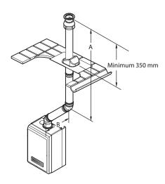
Ø60/100 => Max. length: A+B-(1 x 45°elbow) = 21-1 = 20 m Ø80/125 => Max. length: A+B-(1 x 45°elbow) = 70-1 = 69 m
