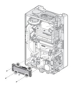
8. With the internal components exposed, locate the gas inlet pipe and the gas valve in the middle of the unit, as shown in Figure 2-1 and Figure 2-2.
