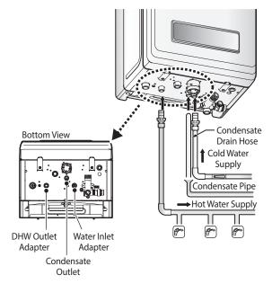
When installing the DHW system, follow these guidelines:
