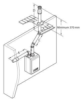
Ø80/80 => Max. length: A+B+C+D-(2 x 45°elbow) = 110-(2 x 1.4) = 107.2 m
