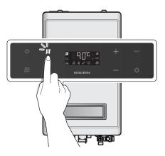
2. Press the + (Up) or – (Down) buttons until the desired temperature appears on the display.
