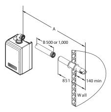
Ø60/100 => Max. length: A=20 m Ø80/125 => Max. length: A=68 m
