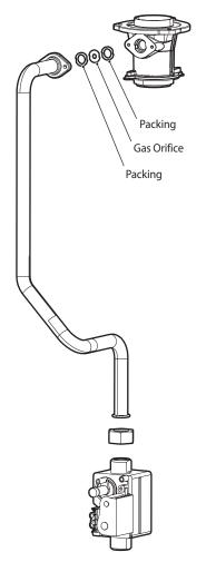
Figure 5-1. Exploded View of Gas Pipe Assembly (NCB-24/28/34LDWE)
