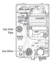
Figure 2-2. NCB-40LDWE Internal Components
