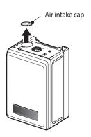
2. Connect the corresponding adapters to the boiler (the gas removal and air intake adapters).
