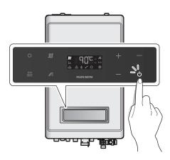
When the power is on, the water temperature of the space heating supply will appear on the front panel display.
