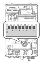
Figure 6. Set the DIP switches
