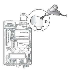
Figure 7. Insert the Analyser
