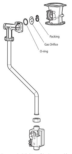
Figure 5-2. Exploded View of Gas Pipe Assembly (NCB-40LDWE)
