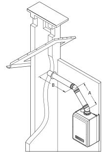
$\emptyset$ 60/100 => Max. length: A+B-(1 x 45°elbow) = 20-1 = 19 m  $\emptyset$ 80/125 => Max. length: A+B-(1 x 45°elbow) = 68-1 = 67 m
