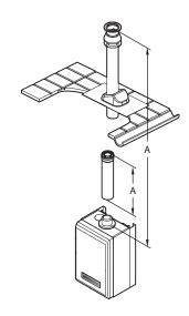
Ø60/100 => Max. length: A=21 m Ø80/125 => Max. length: A=70 m
