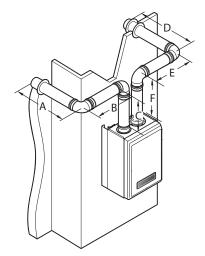
Ø80/80 => Max. length: A+B+C+D+E+F-(4 x 90°elbow) = 110-(4 x 2.2) = 101.2 m
