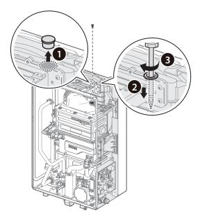
12. Remove the five bolts connecting the mixing chamber and the heat exchanger, and then remove the mixing chamber, burner and the chamber bracket.
