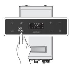
3. Press + (Up) or – (Down) buttons until the desired temperature appears on the display.
