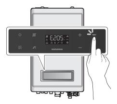
If resetting the boiler does not solve the problem, refer to the Troubleshooting section of this manual or contact Technical Assistance Service.
